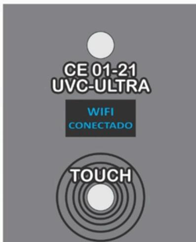
If there is a WIFI network previously registered in the box's internal memory, and if it is within range and available, the box will connect to the network and the success message "WIFI CONECTADO" (WIFI CONNECTED) will be displayed on its screen. The system will then connect to the on-line server to automatically update the internal clock with the date and time. Upon successfully completing the process, the box will begin its initialization cycle.
