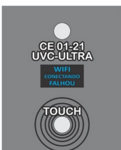
If there is no WIFI network previously registered in the box's internal memory, or if there is one but the box is not within its reach, or if for any other reason the connection is unsuccessful, the message "WIFI CONECTANDO FALHOU" (WIFI CONNECTING FAILED) will be displayed.
