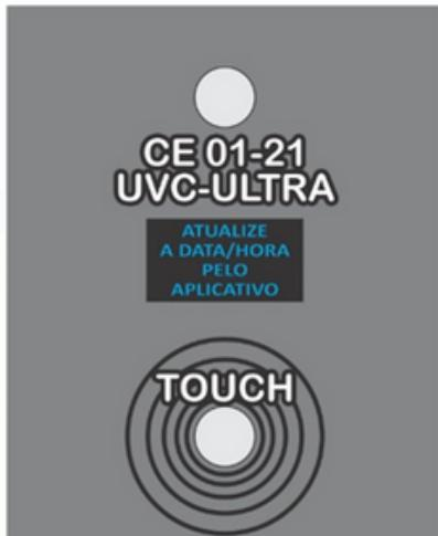
If there is no success in the WIFI connection, or if the on-line server is not accessible even with WIFI connected, the system will not automatically update the internal clock, displaying the following message: "ATUALIZE A DATA/HORA PELO APPLICATIVO" (UPDATE DATE/TIME VIA APPLICATION) requiring the operator to use the application to perform the update. See instructions for the application in the manual.
