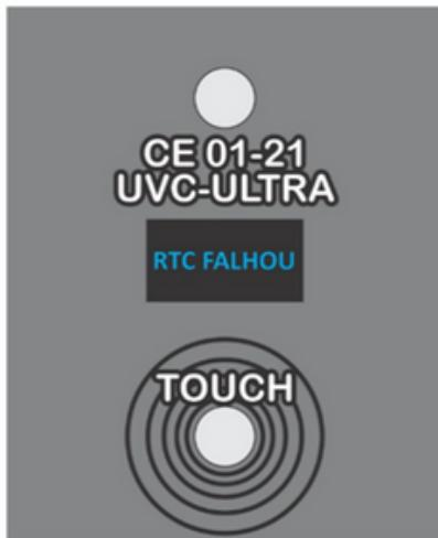
If there is no success in initializing the internal clock, the message "RTC FALHOU" (RTC FAILED) will be displayed and the box will not initialize. In this case, contact technical assistance.
