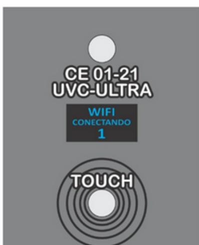
If there is success in initializing the internal clock, the next message to appear is the WIFI connection message. The box will try 5 times to connect to a WIFI network already previously registered in its internal memory by the box's exclusive APP.
