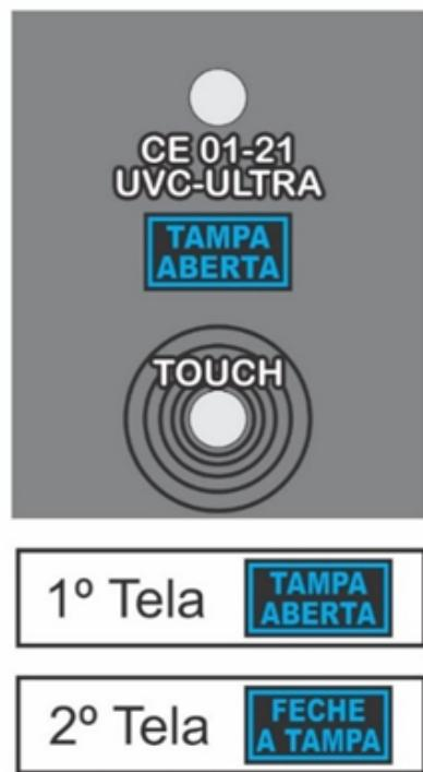
If, after touching the touch sensor, the system identifies that the lid is open or not closed correctly, the following error message will appear on the display: "TAMPA ABERTA FECHE A TAMPA" (LID OPEN CLOSE THE LID). This message will remain until the lid is correctly closed, and the display returns to showing the clock with DATE/TIME, requiring the operator to touch the touch sensor again to restart the sterilization process.
