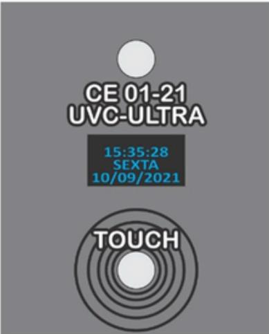
Before starting the sterilization process, the operator must verify the hygiene conditions of the equipment, which must be in accordance with the protocol for the decontamination of surgical instruments. Following all hygiene and preparation recommendations, simply place the instruments to be sterilized on the quartz tray according to the instructions for use, close the box lid, and touch the touch sensor with a finger for the sterilization process to begin.
