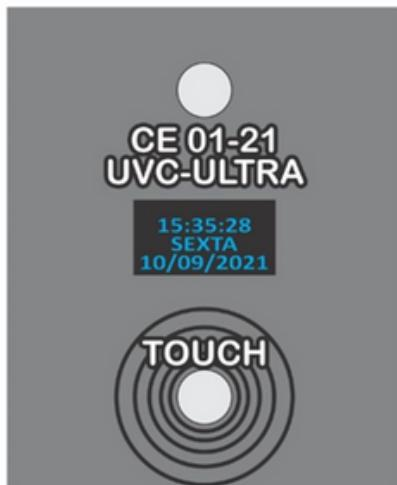
Having successfully loaded all resources, without any error message, the box will display the current DATE AND TIME on its screen, informing the operator that it is ready for sterilization procedures.
