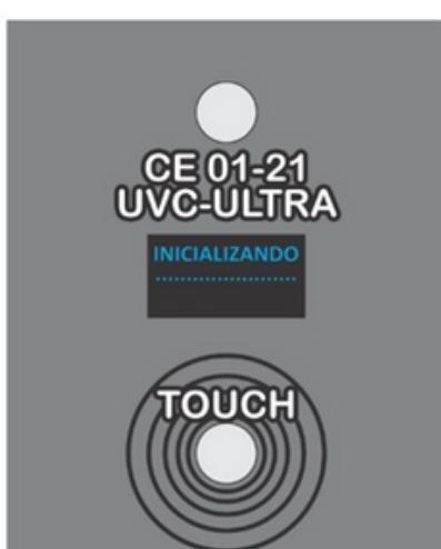
Immediately after the DATE/TIME update automatically performed by WIFI using the on-line server or updating via the application, the system will enter the initialization mode, loading all the box's resources.
